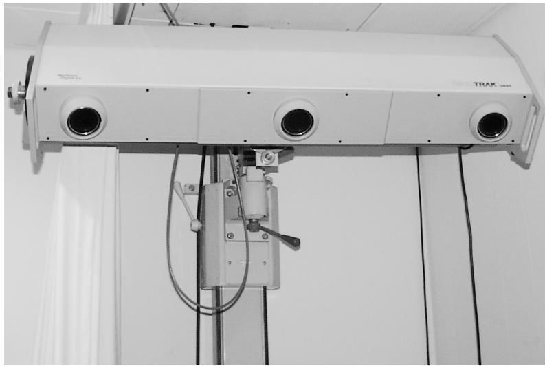
**Figure D.1:** The Optotrak 3020 system that was used to record the grasp trajectories. Clearly visible are the three infrared video cameras. The system is attached to a concrete wall which inhibits vibrations of the cameras.
